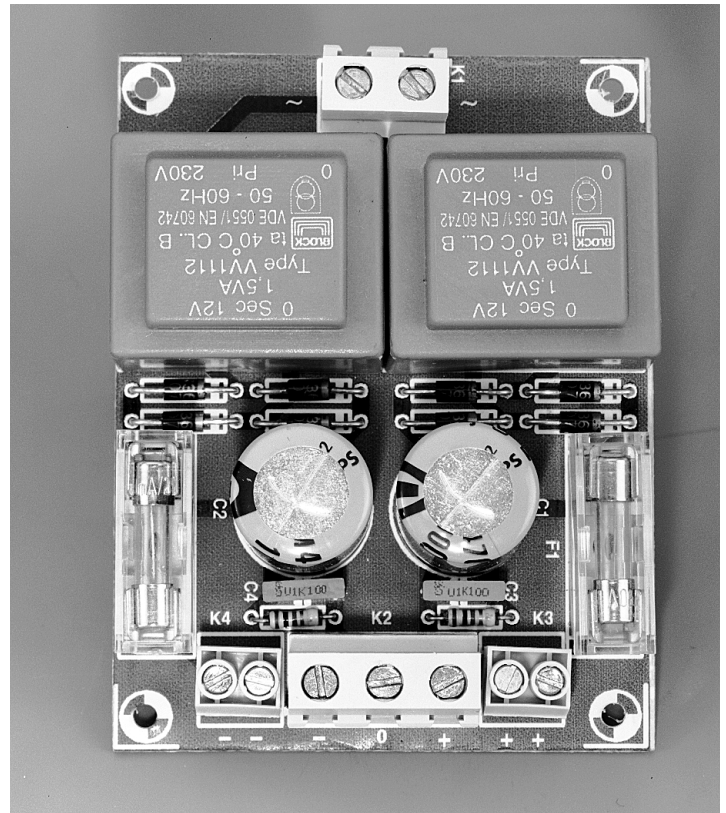
Figure 8. The auxiliary power supply is small enough to fit in most enclosures.
